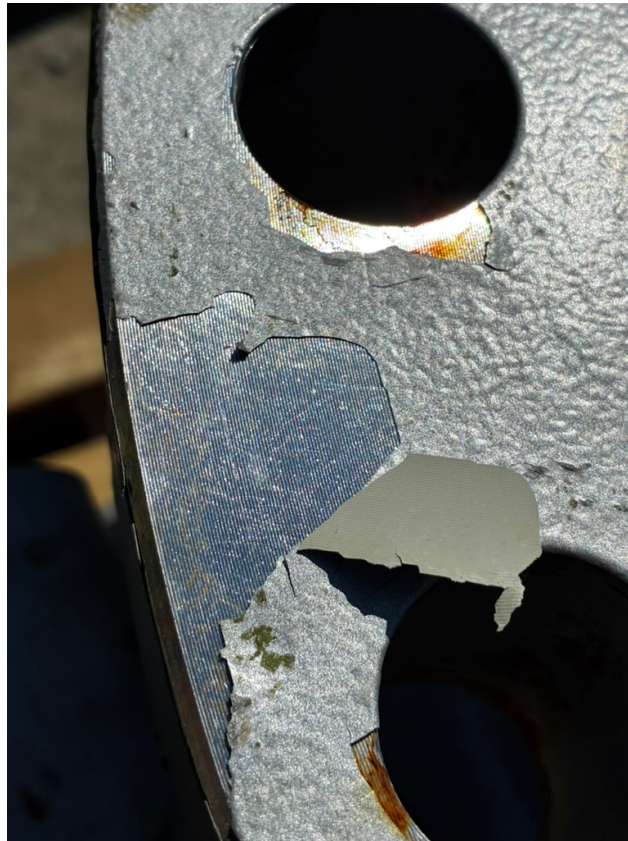
Figure 1. Extensive coating separation from a machined metal surface. Milling/turning marks and locally exposed base metal are visible.
