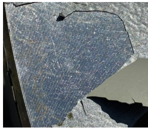
Machining marks and a clean fracture plane
